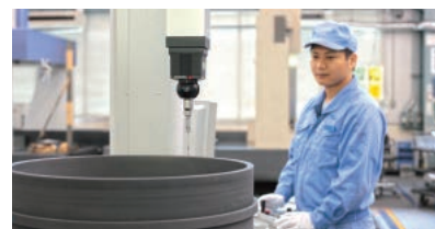
Inspection using 3D measurement machine
