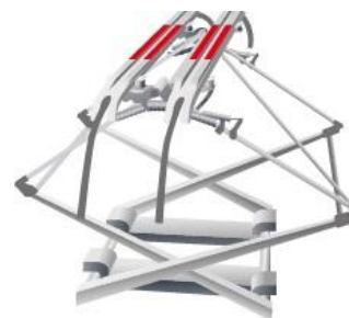
Contact strips for pantograph
